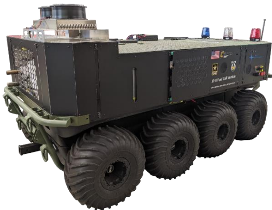
Figure 2: F-24/JP-8 fueled, electric SMET prototype developed at PCI with US ARMY DEVCOM GVSC support. It is self-charging and provides 10-kW e export power.
