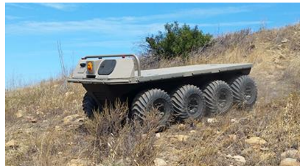
Figure 3: Multi-Utility Tactical Transport developed by GDLS. It requires external charging and provides 3 kW e export power. ( https://www.gdls.com/products/tracked-combat/MUTT.html )
